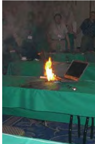
Laptop Battery Fire
