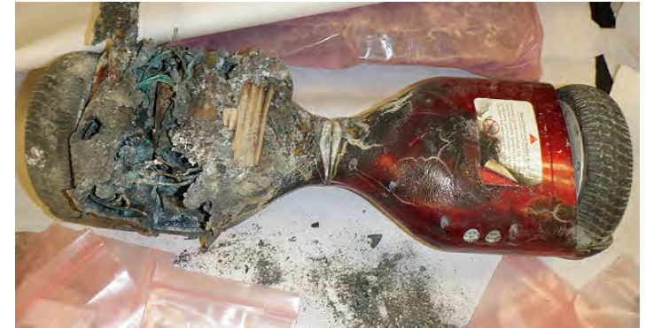
Aftermath of a Hoverboard Battery Fire
