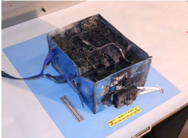
Aftermath of the Boeing Dreamliner 787 Battery
