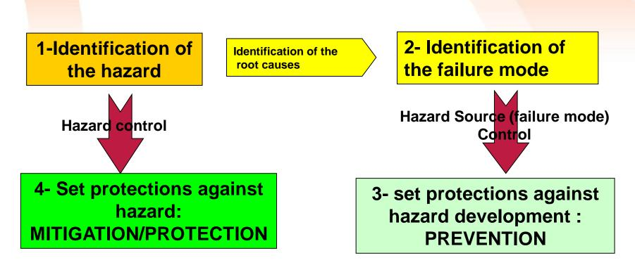
A Hazard analysis is necessary to define the relevant prevention and protection solutions for each application:
