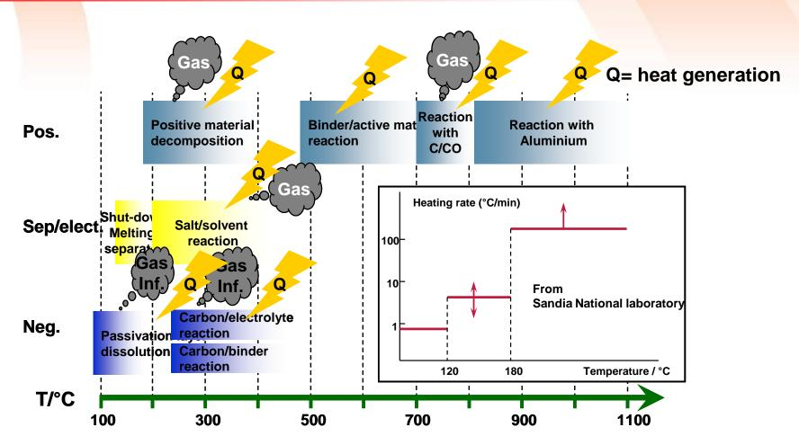
Without appropriate design to limit the thermal run away (such as venting, insulating layers,...), the chain of reaction leads to a violent event.
